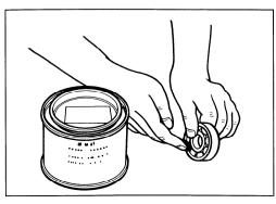
• Install the wheel bearings with the special tool.
